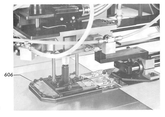
On striped or check materials make sure that the patterns on cutting and pocket blank agree. This can be checked by means of the window in the pocket plate. The operator can determine whether the position of the cutting or of the pocket blank is to be corrected.
