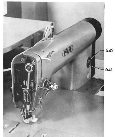
6. FOLD.UT. This button is pressed to lower the folding unit and table insert.
