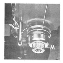
Open the latch of the bobbin case; this stops the bobbin from falling out. Hold the latch open, insert the bobbin case in its base, then release the latch. Press the bobbin case lightly until you hear it snap in place.
